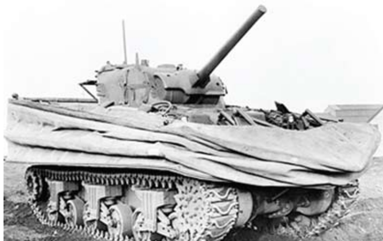
SURF AND TURF Many ideas founder at the border of sea and land. This canvas-sided modification—dubbed Duplex Drive—to make the M4 Sherman tank seagoing, was never seen after World War II.
