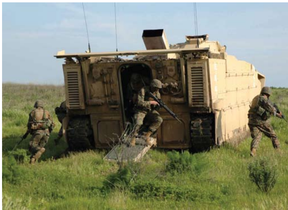
NEEDS BETTER PROTECTION Combat in Iraq and Afghanistan have pointed out a need for better protection for the EFV, shown here in testing. Armor kits for the hull bottom have been proposed.
