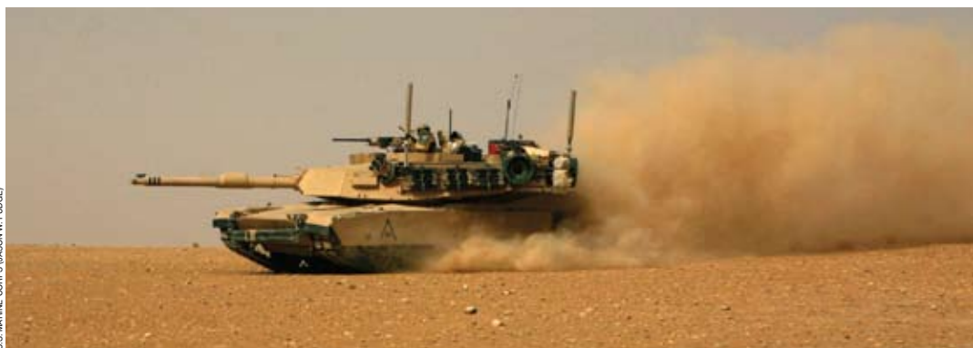
A POWER HOG The EFV’s need for speed on water demands a 2,700-hp powerplant. This is 1,200-hp more than the one used to power the M1 Abrams tank, shown here, which weighs two-thirds again as much as the Marines’ projected vehicle.
